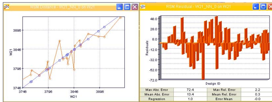
Fig. 12.4. Tools for measuring the quality of meta-models. Distance chart that points out the differences between real values and values calculated using the meta-model, (left) and residual chart (right). The residuals are the amounts which the meta-model has not been able to explain (approximation errors). These charts help to determine whether a meta-model is an acceptable representation of the original problem.
